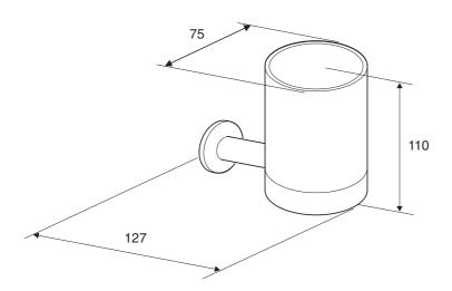
All measurements shown are in millimetres. Sizes are approximate.
